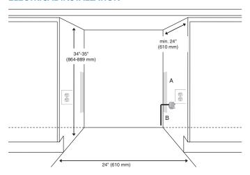
A: Recommended area for installation of power connection – a 2 ½" (63 mm) diameter hole is recommended 3: Location of power cord – approximately 15" (381 mm) from base of appliance
