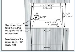
Cabinet dimensions for installations into a cabinet wall. Front of appliance door is flush with the cabinet front surface. Front opening results in a 3/16" gap between appliance door and outer recess.
