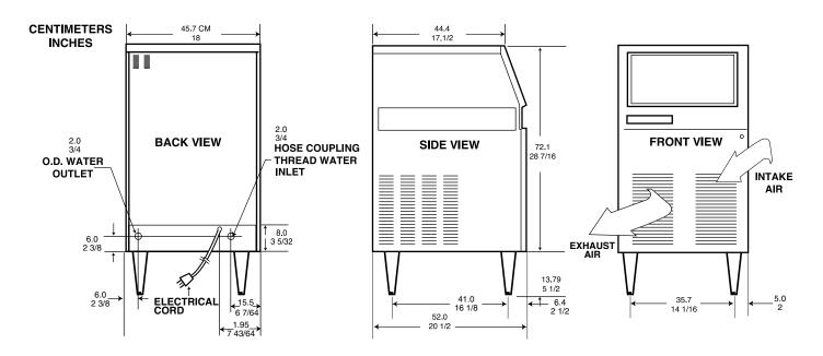
Installation Note: Allow 6" minimum space at back for utility connections
