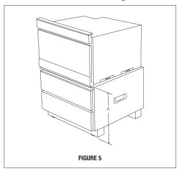
6. Install the wooden cleats. Align the bottom of the cleat to the measurement from Step 5. The pedestal can be installed flush or standard with the face of the cabinet. Depending on the preference, the depth of the cleat position should be adjusted as such. See Figure 6. Position each cleat and mark the holes on the cabinet. Pre-drill each hole in the cabinet using a <sup>1</sup>/16" drill bit. Attach both cleats using the 4 mounting cleat screws. See Figure 7.
