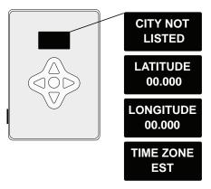
**5.** Setup is now complete. Make sure to keep your Shabbos Keeper in a proper storage location as described in the installation instructions. To adjust the time, date, or location parameters again, hold down the left and right arrow keys for 5 seconds to reset the device.
