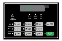
Quantum® Control Features: Digital display for vend price and cycle time countdown. Touch pad control with LEDs.
