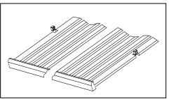
When removing the wooden shelf from the inner rails, make sure to remove all bottles first. Then move the shelf to the position where the potches in the wooden shelf are example.
