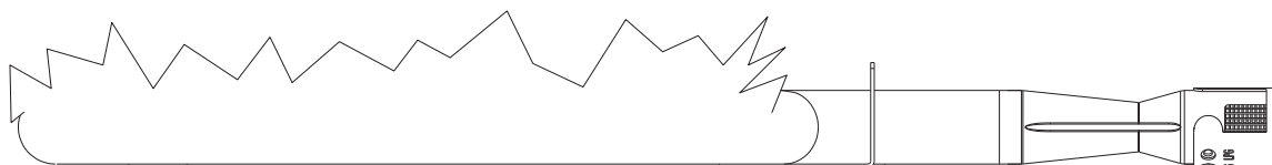
Poor Combustion: wavy, yellow flames-too little air
