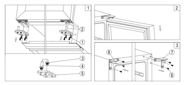
NOTE: All parts removed must be saved to allow the door swing to be reversed.
