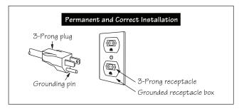
AWARNING Improper use of the grounding plug can result in a risk of electric shock. Do not use an extension cord. If the power supply cord is too short, have a qualified electrician or serviceman install an outlet near the appliance.
