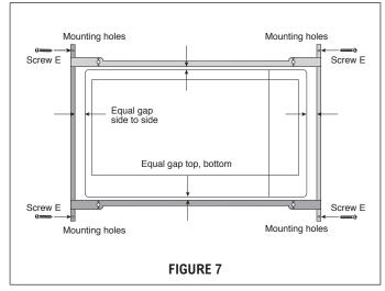
5. FRONT FRAME INSTALLATION: Place the FRONT FRAME onto the BACK FRAME and align ball studs and receivers. Secure the FRONT FRAME to the BACK FRAME by firmly pushing the FRONT FRAME onto the BACK FRAME engaging the 4 snap attachments. See Figures 8 and 9.
