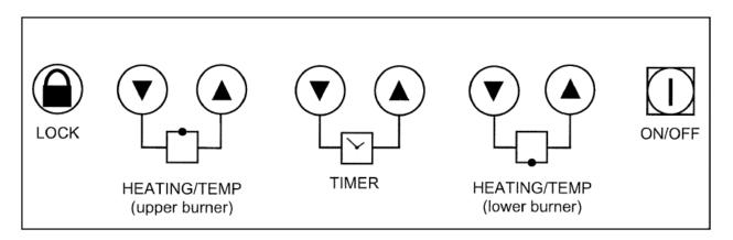
ON/OFF refers to the appliance power, while HEATING/TEMP and TIMER refer to specific functions.
