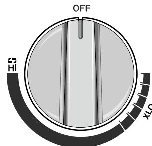
To operate: Select the appropriate control knob, push down and turn counterclockwise until the control knob is set within one of the five XLO settings. Turn off by turning the control knob clockwise to OFF.
