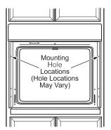
The screws must be a minimum of 6 mm (1/ 4") from the front of the cutout.
