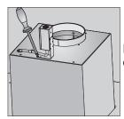
Fix the connector box to the motor junction plate with 2 pieces of 3,5 x 9,5 RYSB screws as shown.
