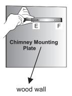
Screw the chimney mounting parts into  $\varnothing$  10mm sized wall plugs on E,F points which is provided with your product.
