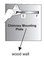
Screw the chimney mounting parts into Ø 10mm sized wall plugs on E,F points which is provided with your product.
