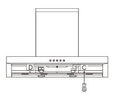
**NOTE:** If the hood seems to be tilting, slightly loosen the screws that are used on the hanging parts at the top and straighten until the hood is vertical.
