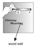
Screw the chimney mounting parts into  $\varnothing$  8mm sized wall plugs on E,F points which is provided with your product.
