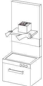
Then fix the body on (A,B) holes to the wall using the screws.
