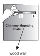
Screw the chimney mounting parts into  $\emptyset$  10mm sized wall plugs on E,F points which is provided with your product.
