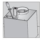
Fix the connector box to the motor junction plate with 2 pieces of 3,5 x 9,5 RYSB screws as shown.
