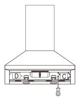
**NOTE:** If the hood seems to be tilting, slightly loosen the screws that are used on the hanging parts at the top and straighten until the hood is vertical.
