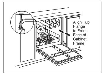
Fasten the dishwasher to the underside of the countertop with the 2 Phillips screws provided.
