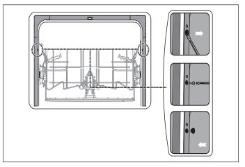
**IMPORTANT** Drive screws straight and flush. Protruding screw heads will scratch the top of the control panel and can interfere with the door's ability to close. If the gap is less than <sup>3</sup>/8" between control panel and the screws, method 2 is recommended.
