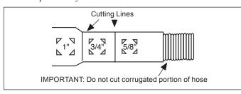
• If a longer drain hose is required, add up to 42" of length for a total of 10 feet to the factory installed hose. Use <sup>5</sup>/8" or <sup>7</sup>/8" inside diameter hose and a coupler to connect the two hose ends. Secure the connection with hose clamps.
