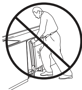
Do not push against front door panel with knee. Damage to the door panel will occur.
