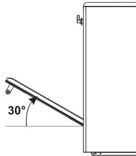
Grasp the door on both sides with both hands, lift it forming an angle of about **30°** and remove it.
