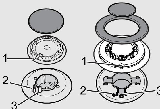
Before lighting the hob burners, make sure that the flame-spreader crowns are correctly positioned in their housings with their respective burner caps. Make sure that the holes 1 in the flame-spreader crowns are aligned with the igniters 3 and thermocouples 2.
