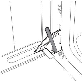
Open the door completely. Insert a pin in the hole in the hinge. Repeat this operation on both hinges.
