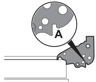
To reassemble the door, put the hinges in the relevant slots in the oven, making sure that grooved sections **A** are resting completely at the bottom of the slots. Lower the door and once it is in place remove the pins from the holes in the hinges.
