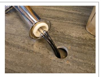
3. Using the 3/8" -thick foam pad included in the tapping kit and roll into a cylinder. From inside the cabinet, insert the foam tube up through the hole in the counter top until it is firmly against the insulation in the dispensing head. Cut away any excess foam that extends into the cabinet that extends into the refrigerator.
