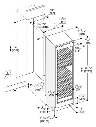
The door face dimensions are designed for a maximum gap of  $\mbox{1/8}\mbox{"}$  (3 mm).
