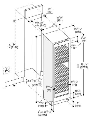
The door face dimensions are designed for a maximum gap of % " (3 mm). See more details on page 247.
