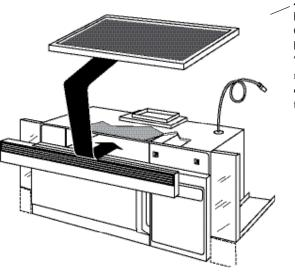
JX81J -RECIRCULATING CHARCOAL FILTER KIT To be used when the microwave oven cannot be vented to the outside.
