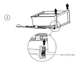
Push the securing tabs on both sides of the bin corners, then push the bin firmly upwards to dislodge from the runners.
