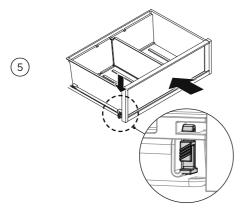
Push the bin slowly onto the securing tabs until you feel it clip onto the runners. Ensure the bin tabs are clipped securely onto the runners before use.
