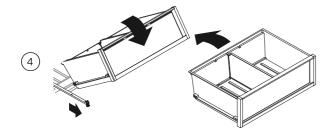
To return the bin, extend the runners and place the bin on top of the runners.
