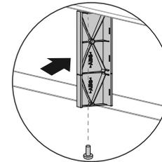
Press the flow divider firmly against the bottom of the door/drawer panel. Ensure the adhesive layer side of the divider contacts the door panel. Secure the air flow divider to the panel with screw.
