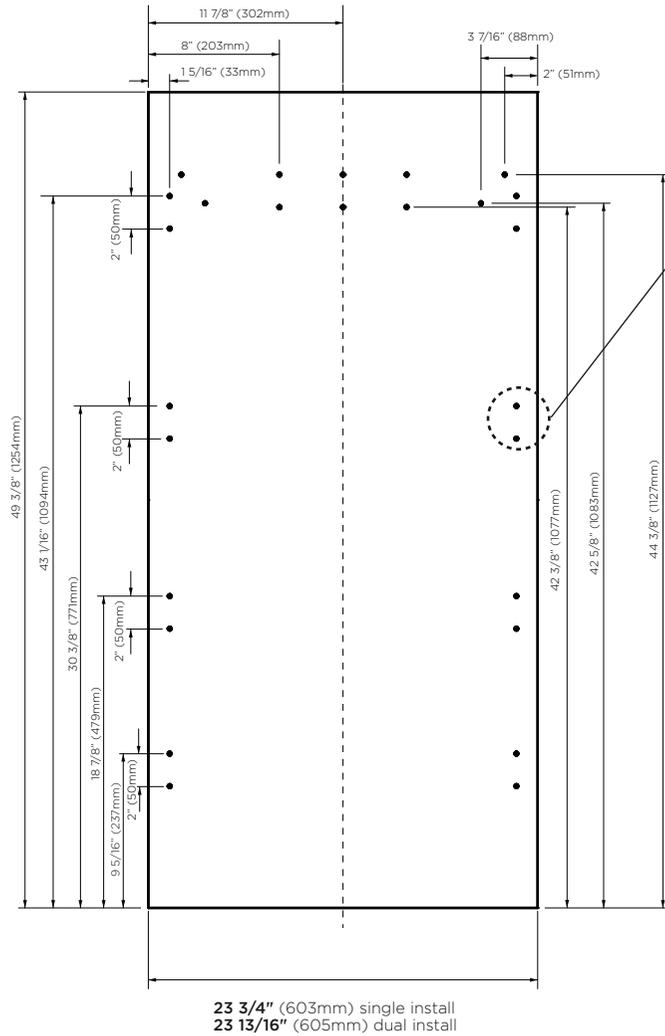
10x Pilot holes recommended for bracket attachment. (Do not penetrate front surface).
