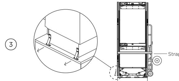
Restrain the appliance with strap and remove the remaining brackets. Use corner posts while strapping to avoid pinching of side trims.
