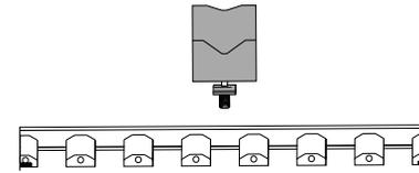
Insert retainer block at desired location between slats of display rack. Do not tighten.
