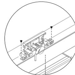
Remove the #8x16 screws (2x) from the sensor housing.
