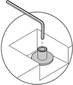
Loosen the M8 screws by 1/8" (3mm).
