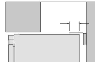
If minimum 7 1/16" (180mm) overlap cannot be achieved, install a solid spacer to the wall stud behind the bracket.
