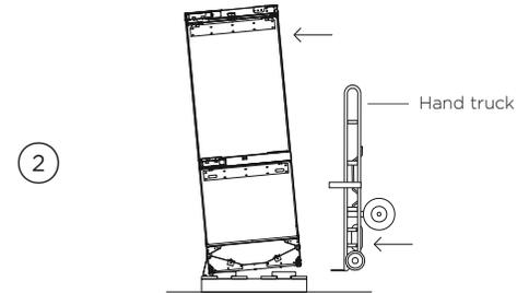
Tilt the appliance slightly forward and insert the hand truck between pallet and appliance.
