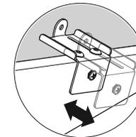
Adjust the brackets to the desired depth by moving it forward/backward.
