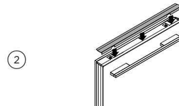
Align top trim to drawer and press down firmly to secure within panel bracket clips.
