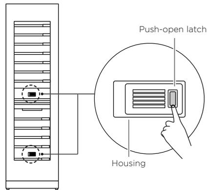
Open the cover of filter housing by pushing the latch.
