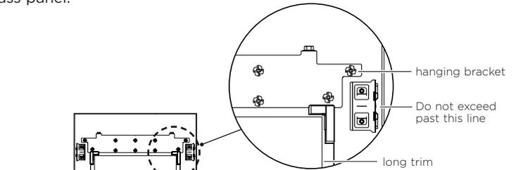
Attach the peeled portion of the trim starting from the top of the door panel cutout.
