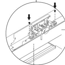
Reinstall the sensor housing using #8x16 screws (2x) into the pre-drilled holes in the cabinet top panel.
