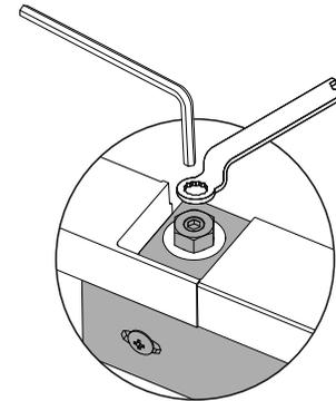
Once satisfied with door panel position, fully tighten M8 washer and nut to adjustment screw.
