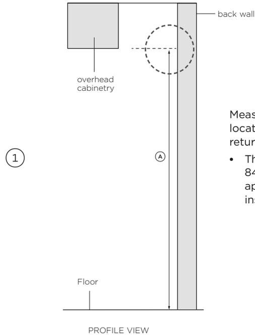
Measure the height (**A**) of the attachment location from the floor to the alcove return.
