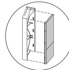
Attach a flow divider cap to the flow divider.
