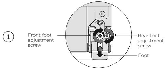
Clockwise turn of the front and rear adjustment screws raise the height of the appliance.
