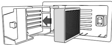
Insert the carbon filter in the hatch.
