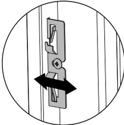
Loosen side screws on the side brackets, and slide door panel forward/backward.
