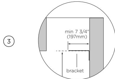
Place the bracket to the backwall. Align the undersurface of the bracket along the marked line.
