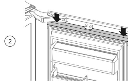
Press down both ends of the top cover to engage the trim caps on the adhesive strips.
