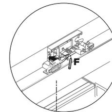
Clip the hall sensor into the sensor housing in the pocket closest to the centreline of the cabinet.
