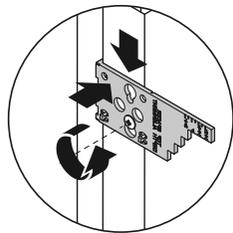
Place the alignment gauge by inserting the screw head through the keyhole of the gauge.
