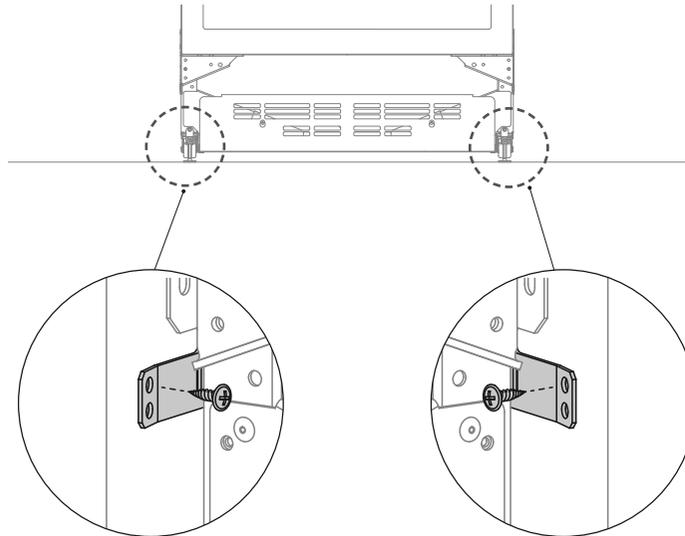
Fix the side brackets (2x) to the lower right and left sides of the cabinetry with 8Gx16 countersunk screws.
