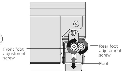
Turn the front and rear adjustment screws clockwise to raise height of the appliances and counter-clockwise to lower the height.
