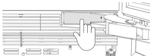
Press the pocket cover to ensure the cover clips into the pocket.
