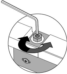
Turn the adjustment screw to raise or lower the height of the door panel relative to the door.
