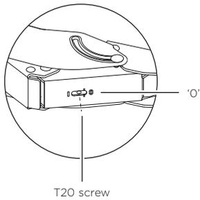
Release the hinge spring by turning the T20 screw in the hinge to the '0' position. Close the door and lay the appliance on its back on the pallet.
