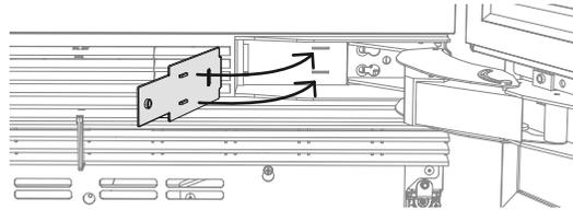
Place the hinge pocket cover to the hinge pocket, matching the studs on the cover to the slots in the hinge pocket.
