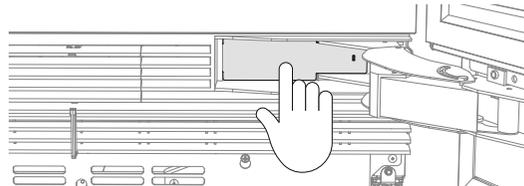
Press the pocket cover to ensure the cover clips into the pocket.
