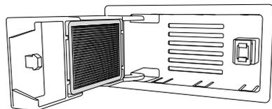
Push the filter gently into the hatch until flush, and then close the cover until it locks to the latch.
