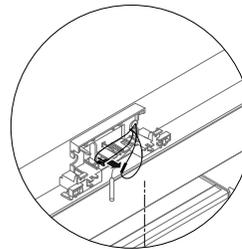
Unhook the interceptor board harness from sensor housing so harness is loose.
