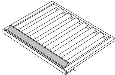
Align handle to the front end of display rack.
