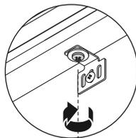
Re-tighten the screw at the bottom of the door.
