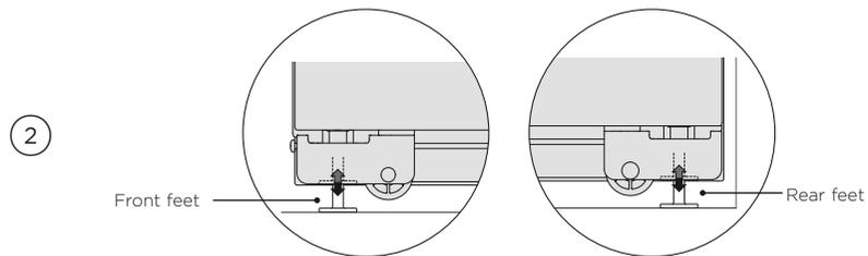
Turn the front and rear adjustment screws clockwise to extend the front feet and rear feet until they engage the floor and the top bracket reaches the cabinetry ceiling.
