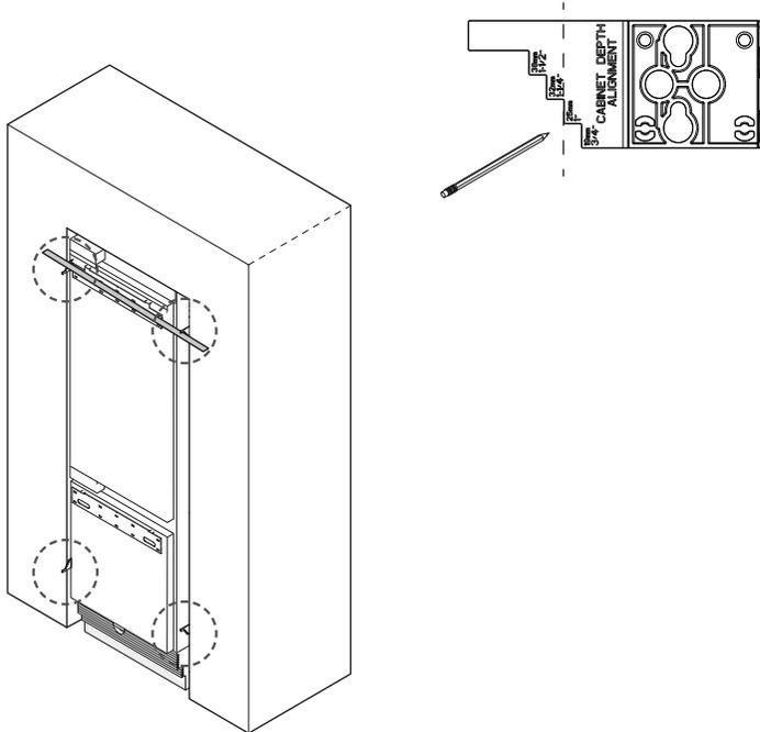
On the 'Cabinet depth alignment' side of the depth gauges, mark the step on both sides of the door based on the thickness of the door panel.
