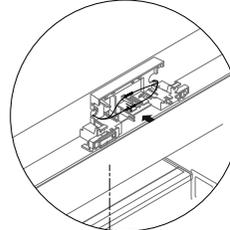
Press the harness from the interceptor board into the forks on the sensor housing.
