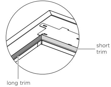
Attach the peeled portion starting from one end of flange perpendicular to top end of long trim.
