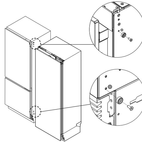
Remove bolts from the locations marked via the green labels on your appliance. Add the flange joiners, and tighten using a 1/8" (3mm) Allen key to secure.
