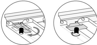
Rotate retainer block to lock position and tighten screw to lock handle in place.
