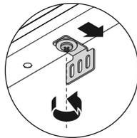
Loosen the screw at the bottom of the door, and slide the locking bracket out until it touches the panel.
