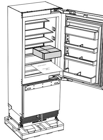
Remove the installation kit and miscellaneous items kit from inside the appliance.
