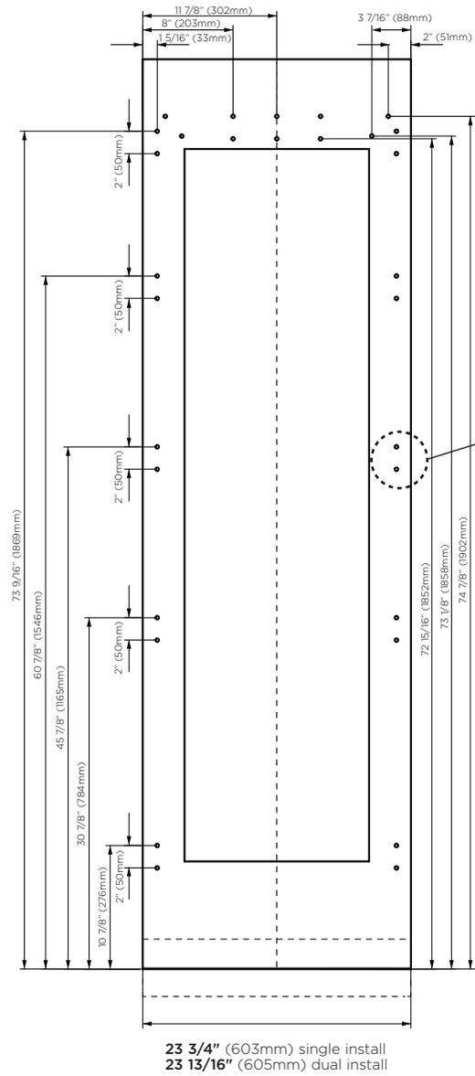
22x Pilot holes recommended for bracket attachment. (Do not penetrate front surface).
