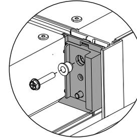
Clamp the upper brackets together by fitting the first the supplied M5 bolt and joiner sleeve. Tighten using a 5/16" (8mm) socket and Phillips screwdriver until the sleeve sits flush.
