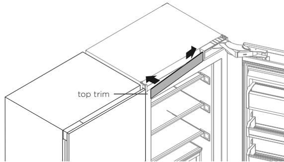
Slide one end of the top trim into the hinge pocket of the appliance.
