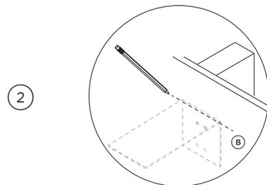
Mark a horizontal line (**B**) at the back wall.
