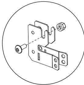
Clamp the lower brackets together using the supplied M6 screw and Nut. Secure using a 3/16" (4mm) Allen key and 3/8" (10mm) spanner. Ensure brackets are clamped tightly before proceeding.
