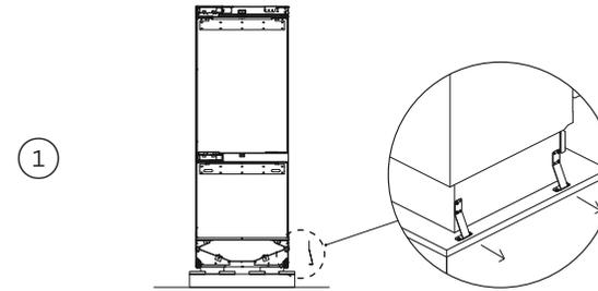
Remove the brackets from the non-hinge side of the pallet.
