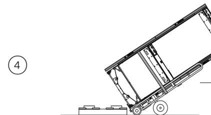
Tilt backward to load the appliance onto the hand truck and set aside the pallet.
