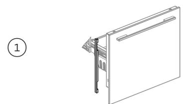
Insert the drawer side covers into the panel gaps on the right and left sides of the drawer. Ensure the cabinet is centered to prevent the side covers from interfering with the cabinet.
