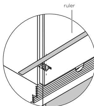
Check the alignment gauges while adjusting the screws to maintain the alignment of the appliance.
