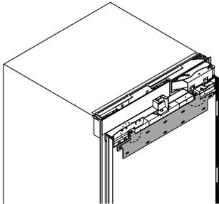
Remove the M8 nut and M8 washer from the M8 screw at the top of the door using the supplied hex key and spanner.
