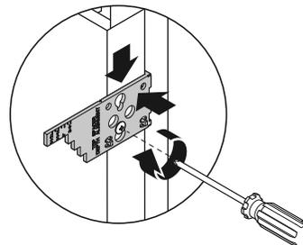
Loosen the right and left screws at the top and bottom sides of the door.
