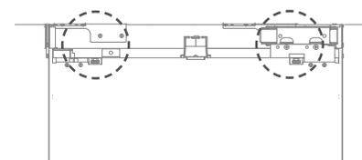
Fix the left and right top brackets to the ceiling surface of the cabinetry with 8Gx16 countersunk screws.
