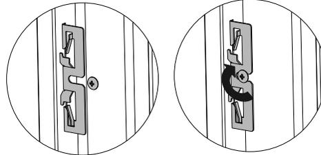
Align the door panel straight with the door and slide-in the side brackets to the side screws of the door,
