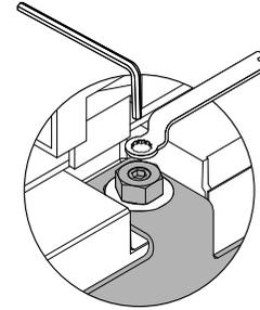
Screw the M8 washer and nut to the adjustment screw and loosely tighten.
