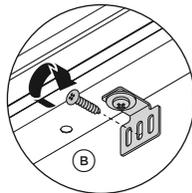
Fix the locking bracket to the door panel with 8Gx16 countersunk screw.
