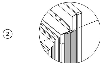
Ensure side cover is aligned with the top door panel extrusion.
