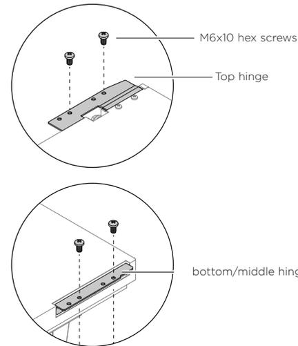
Detach the door from the appliance by unscrewing the door hinge M6x10 hex screws (4x) at the top hinge and bottom/middle hinge.
