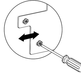
To adjust the door panel further, loosen the M8 washer and nut and slide the door panel to suit. If further adjustment is still required, remove the door panel then loosen the fixing screws of the hanging bracket and move bracket sideways to suit.
