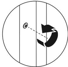
Loosen the right and left screws at the top and bottom sides of the door. Locate the alignment gauges at correct orientation to the right and left screws.
