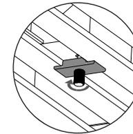
Rotate the retainer block to lock position, and tighten screw.
