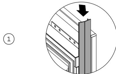
Insert door side covers into the gaps on the right and left sides of the drawer and slide downwards to clip into place. Press firmly to secure.
