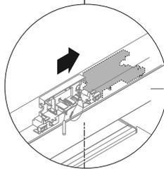
Move the sensor housing to align the opposite hall sensor clip with the centre of the cabinet.
