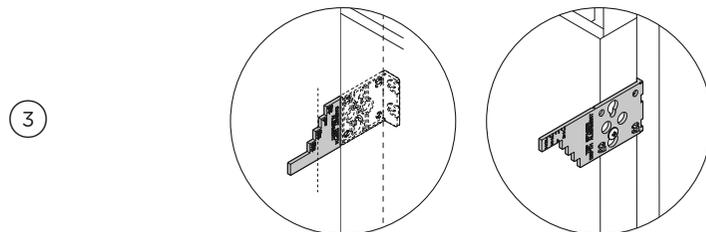
Check the depth gauges while adjusting the screws to maintain alignment of the appliance.
