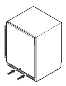
Keep ventilation openings, in the appliance enclosure or in the built-in structure, clear of obstruction.
