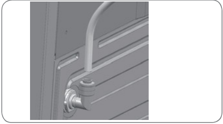
Step 3 ) Connect the PE soft tube.
