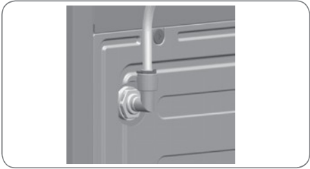
Step 4 ) Install the security clamp.
