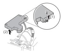
**3** Remove the cover and pull out the tube (1). Disconnect all wire harnesses (2). Unscrew the ground wire (3).
