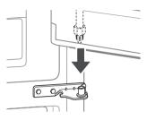
2 Fit the hinge (1) over the hinge lever latch and slot it into place. Rotate the lever (2) counterclockwise to secure the hinge.
