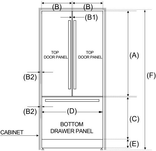
NOTE: The refrigerator comes with a 4" (100 mm) stainless steel toe kick installed to fit a standard 84" (2134 mm) tall cabinet niche. For different toe kick heights, adjust C accordingly. For flush installation in a standard 25" (635 mm) deep cabinet niche, maximum custom door panels thickness is 3/4" (19 mm).
