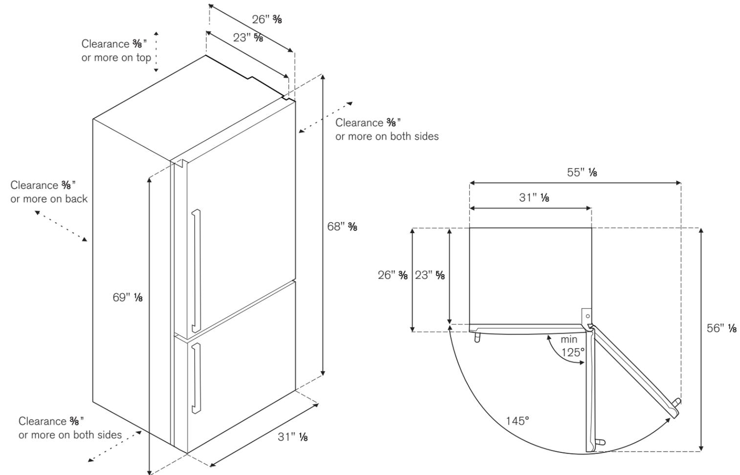
**INSTALLATION:** There shall be a space not less than 3/8 inch from the top of your refrigerator, not less than 3/8 inch from both sides and 3/8 inch or more from the back of the refrigerator to the adjacent walls respectively. This requirement is necessary to create clearance in order to open and close the door as well as to avoid the spacing for adequate ventilation around the refrigerator.
