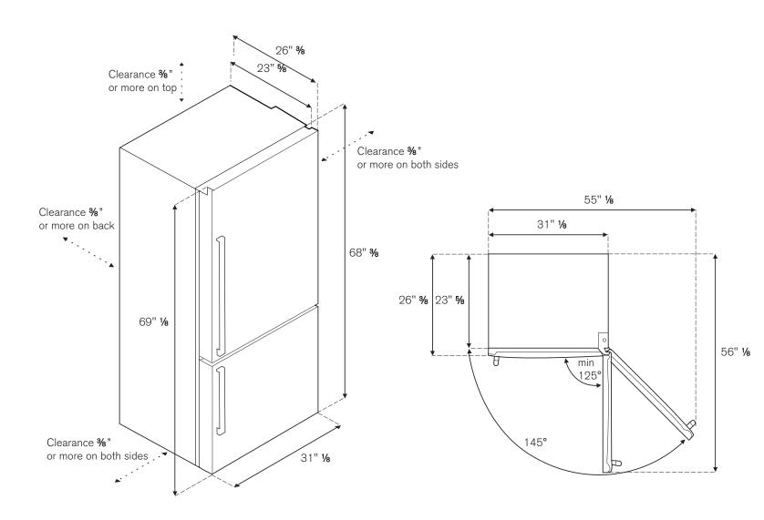
INSTALLATION: There shall be a space not less than 3/8 inch from the top of your refrigerator, not less than 3/8 inch from both sides and 3/8 inch or more from the back of the refrigerator to the adjacent walls respectively. This requirement is necessary to create clearance in order to open and close the door as well as to avoid the spacing for adequate ventilation around the refrigerator.
