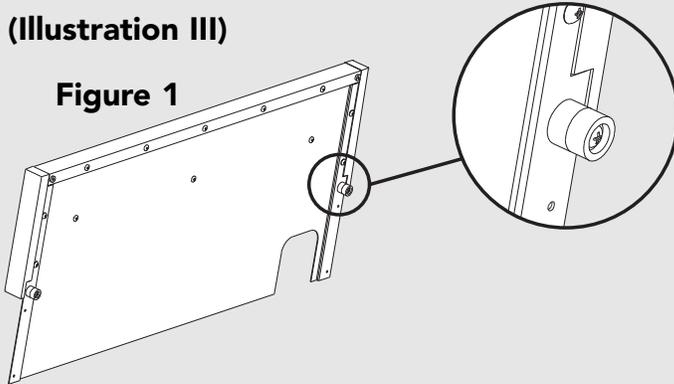
**Note: If the back wall is Non-Combustible, these spacers can be removed. (See Figure 2)**
