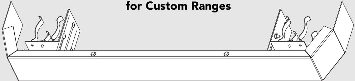
**Important Note:** The range must be installed as specified in the range installation guide for proper airflow when using the standard curb base.
