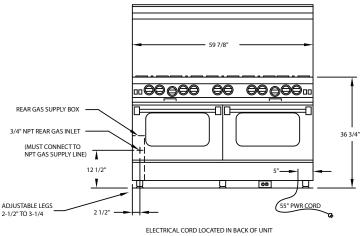
ELECTRICAL CORD LOCATED IN BACK OF UNIT LOCATION OF ELECTRICAL OUTLET MUST NOT BE HIGHER THAN 3" FROM FLOOR IF LOCATED BEHIND THE UNIT OR CAN BE LOCATED IN AN ADJOINING CABINET.
