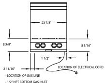
(MUST CONNECT TO NPT GAS SUPPLY LINE)
