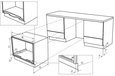
An internal shelf can be used as an alternative to spacer blocks to position the product at the correct height. In this case additional cutouts will be required. Refer to complete installation instructions.
