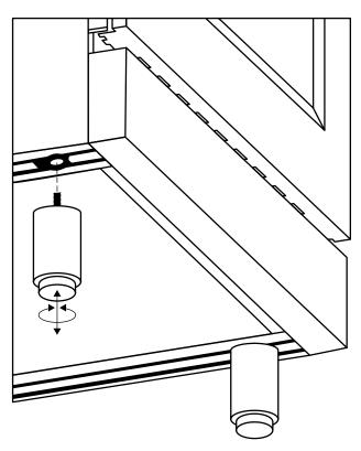
1. Before installing the legs, position the appliance near its final location as the legs are not suitable for moving the appliance over long distances.
