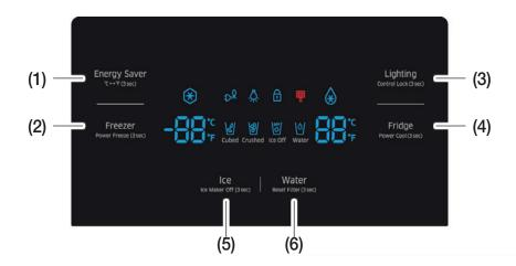
(1) Energy Saver (°C↔°F (3 sec)) For better energy efficiency, press the Energy Saver button.
