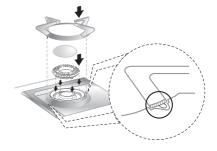
CAUTION: refit all flame caps in the same points from which they were removed. In fact, the flame cap positions cannot be changed. After refitting them, ensure that they are fitted perfectly and that there is no clearance between the top and the flame caps.
