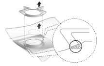
Connection to the gas mains may be made with a flexible metal pipe and conforming to the provisions defined by current standard regulations in force. USE A SOAPY SOLUTION TO CHECK FOR PROPER TIGHTNESS.
