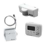
The DigiSmart Occupancy Sensor completes the in-room equipment. This infrared sensor can determine if the room is occupied or empty, and when empty signals the PTAC to adjust the temperature to save energy based on programmable setbacks.
