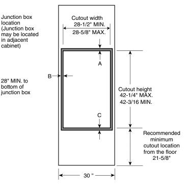
NOTE: If the cabinet does not have a solid bottom. two braces or runners must be installed to support the weight of the oven. For single ovens, the runners and braces must support 200 lbs (91 kg). For double
