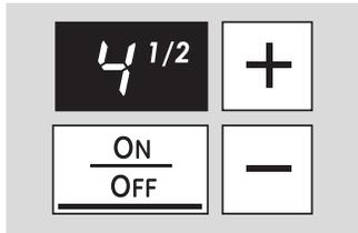
The power level with a fraction indicates the additional half-step setting. You may hear clicking sounds indicating the control is maintaining your desired setting.
