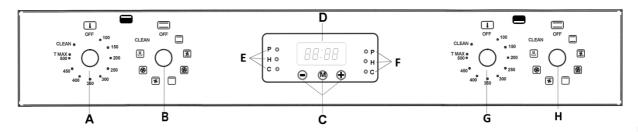
A Temperature knob for lower cavity
