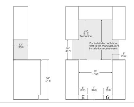
NOTE a.Electrical Connection b.Gas Connection
