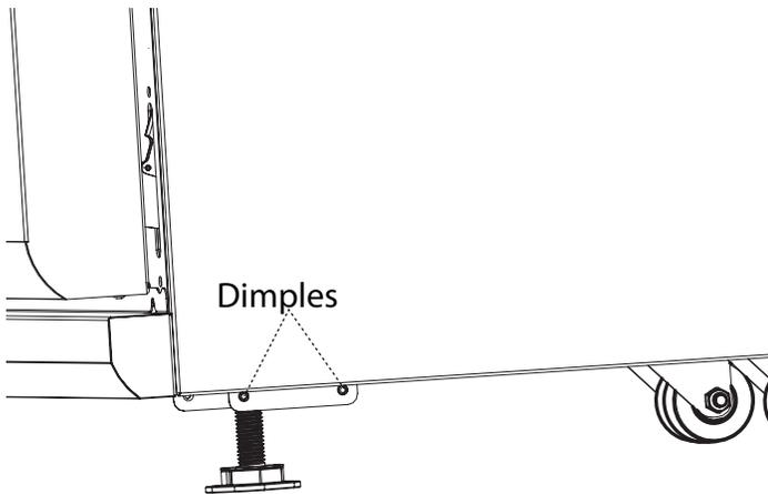
5. Secure the cover assembly through the dimpled holes with (2) 1/2" stainless steel Torx head screws (included), as shown below.
