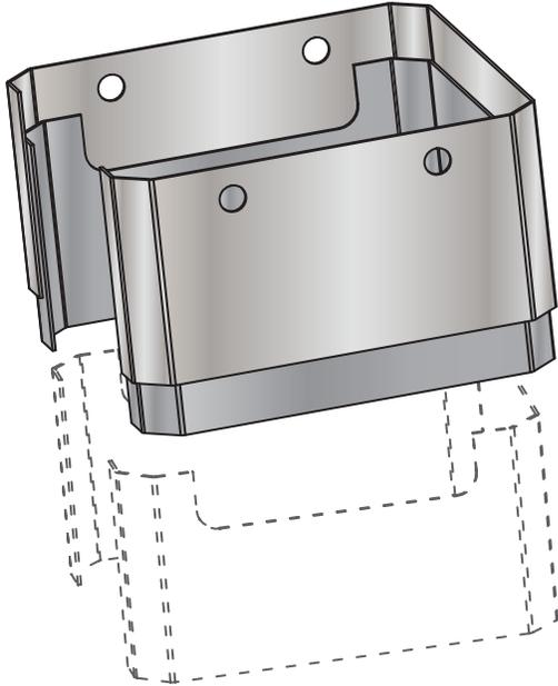
3. Beneath the range, wrap the cover assembly around the leg.
