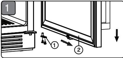
1. Take out the 2 screws from the lower door axis (1), remove the door (2), and the axis plate (1) from the door.
