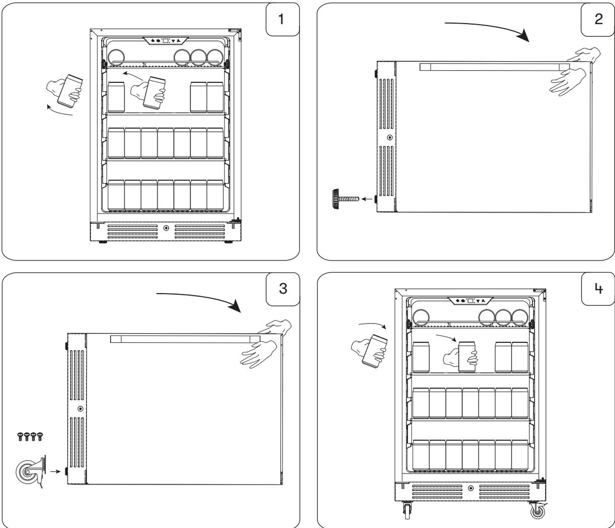
1. Empty all contents within the outdoor beverage cooler and close the door afterwards. Lay the unit gently down on its right side.
