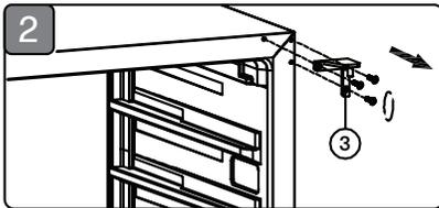
2. Take out the 3 hinge screws from the top right hinge (3) and remove it.
