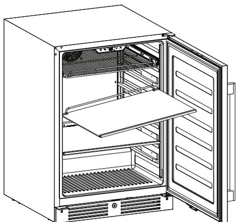
3. Pull the shelf outward until it is removed from the inner compartment. You may encounter some resistance from the shelf guard rail.
