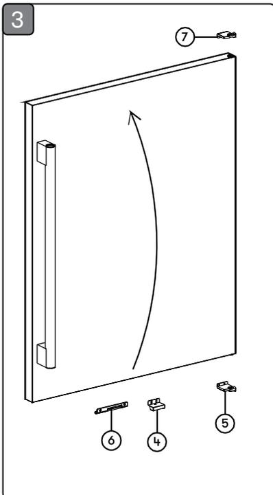
3. All located at the bottom of the door, remove the door magnet (4), door stopper (5), and child safety lock (6) by 2 screws each. Then, install the door magnet, child safety lock, and new door stopper (7) on the opposite side of the door frame. Rotate the door 180 degrees.
