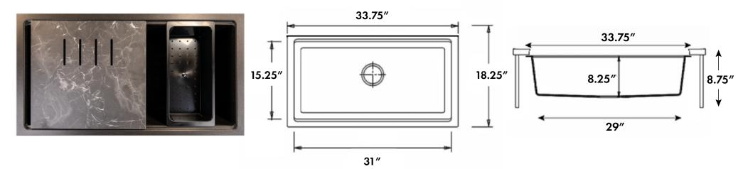
Overall DimensionsInterior BowlExterior BaseInterior DepthDrain Dimensions33.75"x18.25"x8.75"31"x15.25"x7.75"29"x13.25"8.25"3.5"
