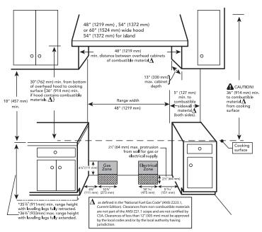
**NOTE:** A 36-inch minimum clearance is required between the top of the cooking surface and the bottom of an unprotected cabinet. A 30-inch clearance can be used when the bottom of the wood or metal cabinet is protected by not less than 1/4 inch of a flame retardant material covered with not less than No. 28 MSG sheet steel, 0.015 inch (0.4 mm) thick stainless steel, 0.024 inch (0.6 mm) aluminum, or 0.020 inch (0.5 mm) thick copper.
