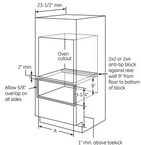
1" min. above toekicl or adjust to oven installation height
